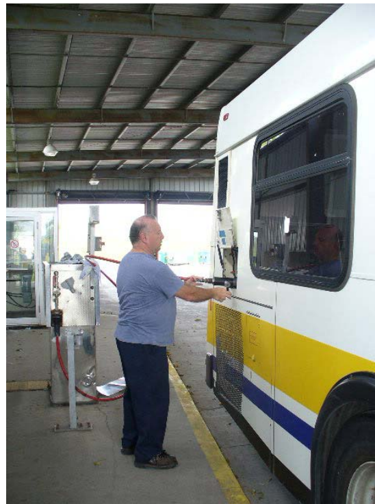
CNG bus refueling at HSR bus garage
